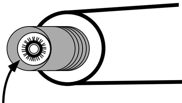
Inside of the connection piece, there is a flow-restrictor that can get filled with fine sand or dirt. Rinse out the dirt. If the black rubber o-ring is removed for cleaning, it must be replaced to meet California flow requirements.
