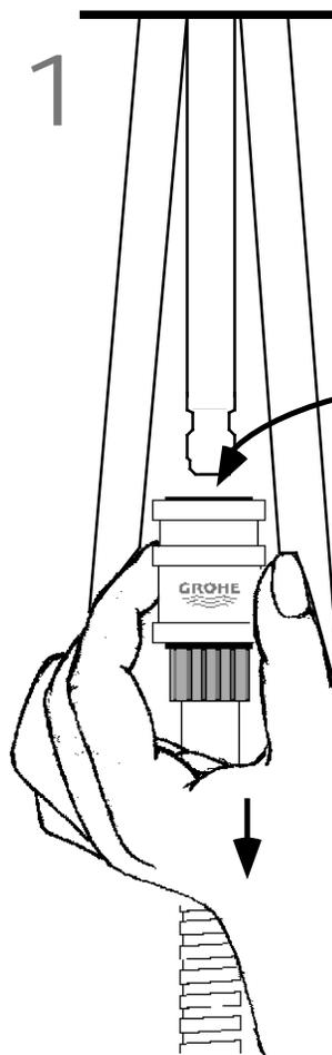
Look under the sink and locate the yellow & black quick coupling. Pull-down on the yellow ring, and the quick coupling will detach from the mixed water supply tube.
